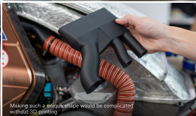
End-cap connectors, a moving part made with Resin Flex
